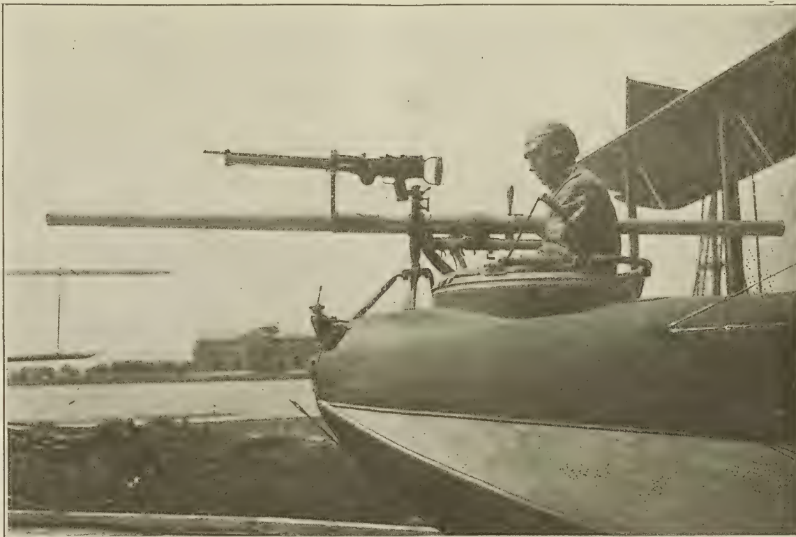
The Davis Non-Recoil Gun was used by the Navy for anti-submarine work, as it is the only gun of large caliber which has been successfully mounted on an airplane. The mounting of a Lewis machine gun to fire tracer bullets is a recent innovation.
